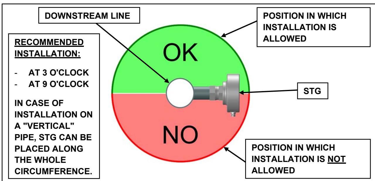
STG has to be installed at the outlet of a safety valve, or in the case of a circuit with multiple valves, it can be mounted on the general downstream manifold line.
